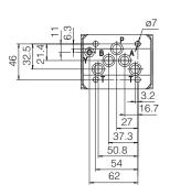
P = PRESSURE PORT A, B = USE PORT T = TANK PORT Y = DRAIN PORT
