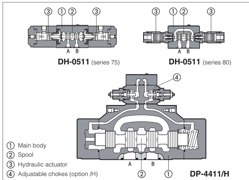
Hydraulic operated directional valves, spool type, three or four way, two or three positions. Available with single or double hydraulic actuator.
