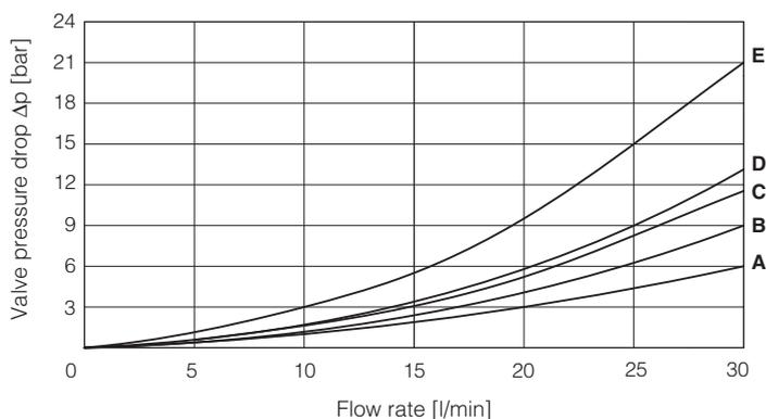
**9 OPERATING LIMITS** based on mineral oil ISO VG 46 at 50°C
