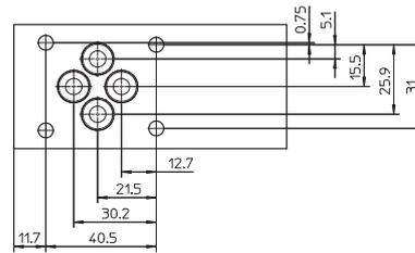
Installation dimension with QVHZO proportional flow control valve and CART M-5 pressure relief cartridge
