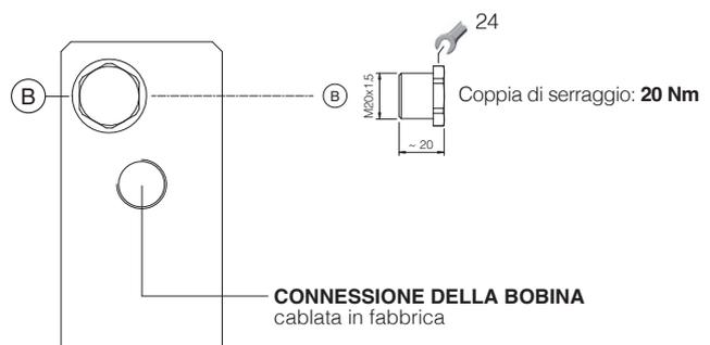
CONNESSIONE DELLA BOBINA
